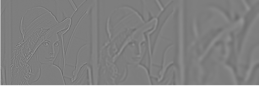
Fig. 5. Fast implementation of LoG operator at scales one, five, and seven using cubic B-spline.
